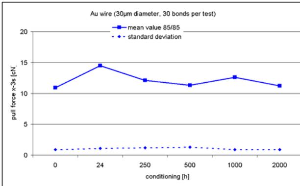
**Fig. 6** Average wire pull forces for gold wire bonds following heat (85°C) and humidity (85%) conditioning
