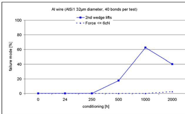
**Fig. 13** Second-bond wedge lifts and average pull forces ≤ 6 cN for aluminum wire heat (85°C) and humidity (85%) conditioning
